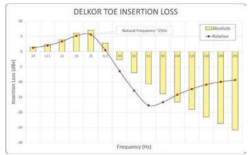
Relative Insertion Loss Reference Track – 150kN/mm
